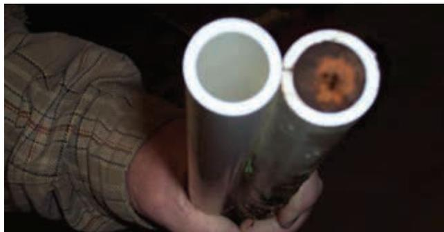
Biofilm (right) causing restricted water flow
